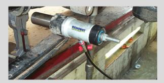
Removing the old bush and inserting a new on a DAF CF85 truck by the use of a EBH18 - kit simply the work. The operation can be performed in a safe and rapid manner.
