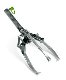
The smaller sizes, 5 ton and 10 ton, are equipped with special mechanics which self centers the arms. The arms will therefore always adapt to the diameter of the object and have the best possible grip and handling. All REHOBOT pullers are furthermore self straining and have an extra long stroke. The pull depth can easily be adjusted by moving the arm attachments.
